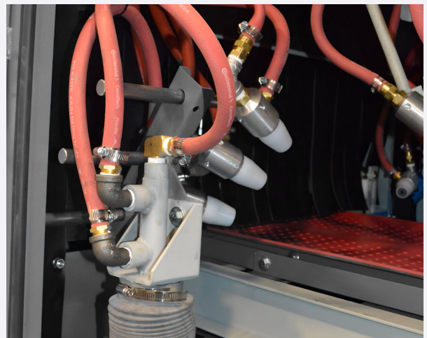
FIX OR OSCILLATING NOZZLES TO COVER BOTH SIDES OF MOVING PARTS
