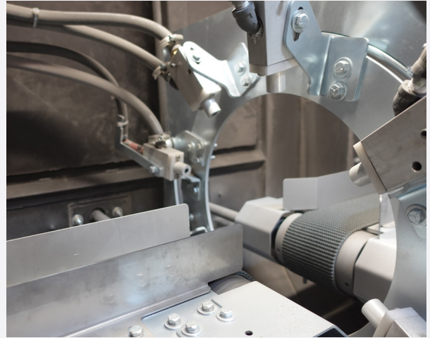
CIRCULAR OSCILLATING NOZZLES ON RING FOR 360 COVERAGE
