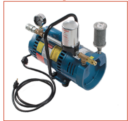
¾ hp Electric Powered Ambient air pump Capacity 10 cfm @ 10 psi
